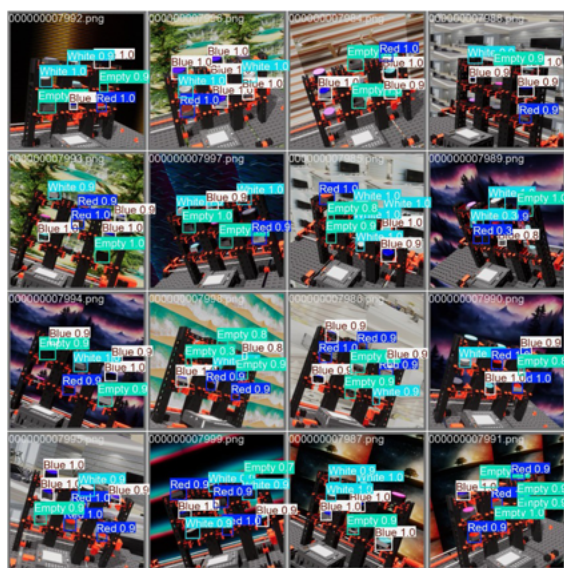
Figure 4: Synthetic data generated by the digital twin.
